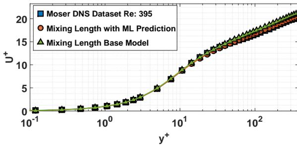
Figure 5: Comparison between the mean flow solution obtained with a predicted correction parameter, against the base mixing length model, and the DNS dataset, at a friction Reynolds number of 395.
