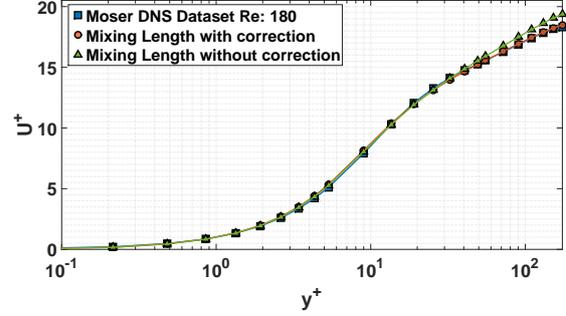
Figure 2: Comparison between Moser DNS data, and the base and corrected models, at a friction Reynolds number of 180.
