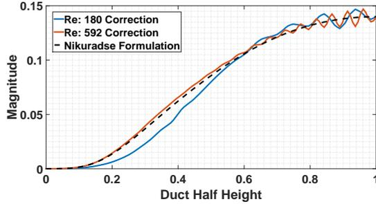
Figure 1: A comparison between the base model mixing length formulation (defined in equation 5), and those learned from a Bayesian inversion scheme using the DNS data of Moser et al.
