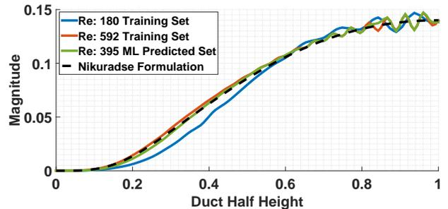
Figure 4: The mixing length curve predicted at a friction Reynolds number of 395 by a regression tree.
