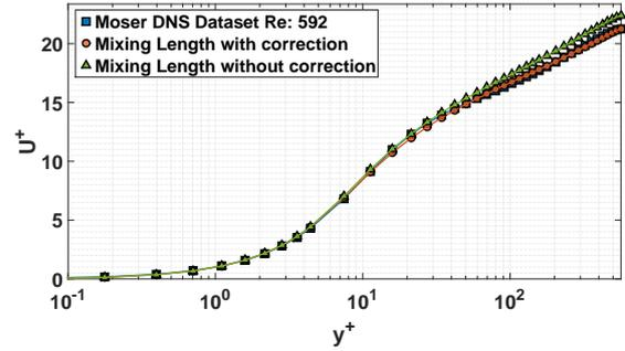
Figure 3: Comparison between Moser DNS data, and the base and corrected models, at a friction Reynolds number of 592.
